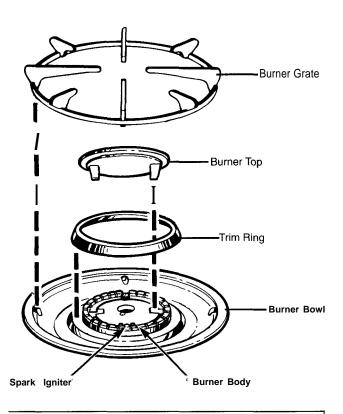
CAUTION: DO NOT OPERATE THE BURNER WITHOUT ALL BURNER PARTS IN PLACE.
